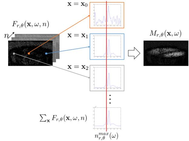
Fig. 5. Procedure for obtaining the vibration modes
