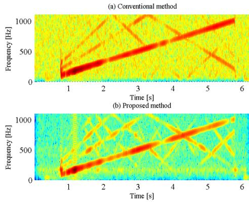
Fig. 9. Spectrogram of sound recovered from object 1
