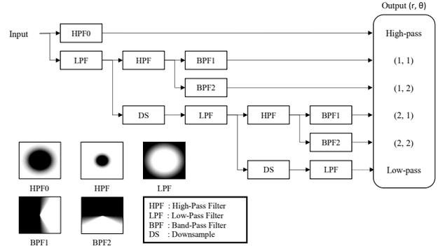
Fig. 1. Procedure of image decomposition using complex steerable pyramid  $(r, \theta) = (2, 2)$
