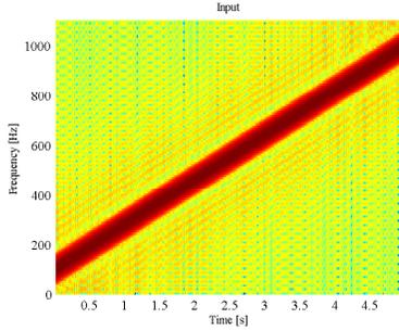
Fig. 7. Spectrogram of input signal (chirp)
