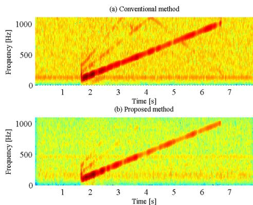
Fig. 11. Spectrogram of sound recovered from object 3
