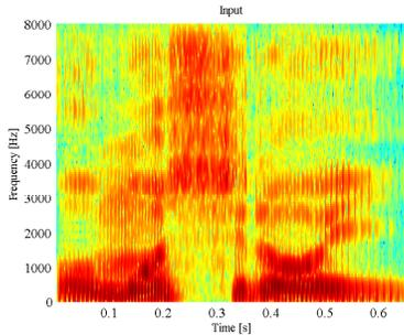
Fig. 8. Spectrogram of the utterance of /o m o s h i r o i/
