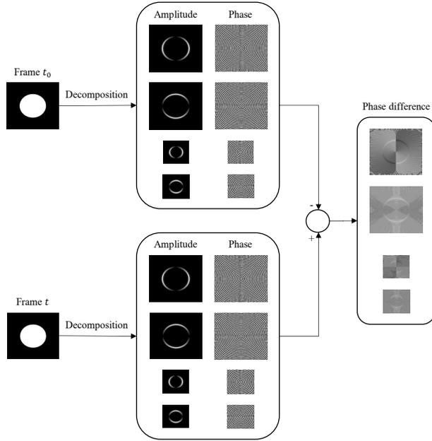
Fig. 3. Procedure of extraction of phase variation
