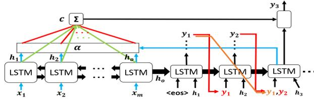
Fig. 3. The attention-based LSTM encoder-decoder model for question keyword class estimation. The encoder is a bidirectional LSTM, and the decoder is a unidirectional LSTM.
