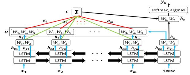
Fig. 2. The *attention-based bidirectional LSTM* model for *question type* estimation. Because, the last state of the forward and backward layer where  $\langle \text{eos} \rangle$  is entered has information of the entire input sentence, it is useful for estimating *question type*.
