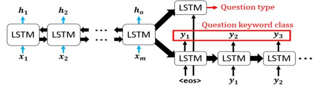
Fig. 4. The joint model. In this model, the question type estimation model and the question keyword class estimation model share the encoder and the attention mechanism.
