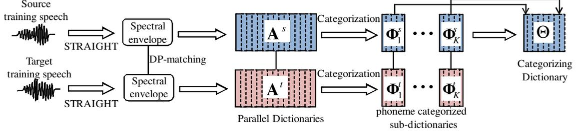
Fig. 3. Construction of categorizing dictionary that consists of representative vectors from each sub-dictionary.
