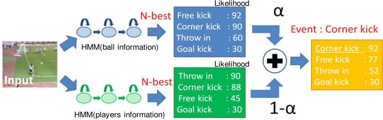
Figure 7. Flow of the result integration method using two types of HMM
