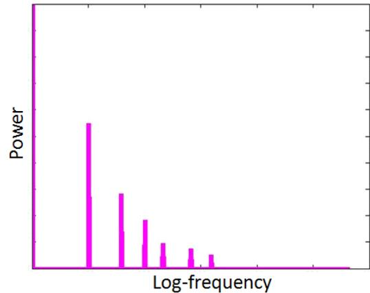
Fig. 3 Example of harmonic structure (piano A3)
