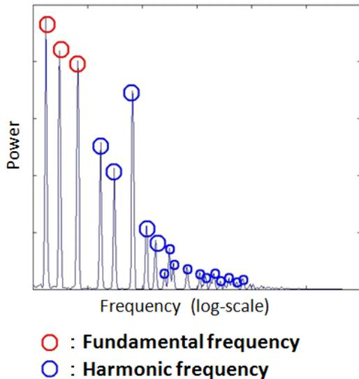
Fig. 2 Observed spectrum (piano triad)
