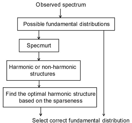
Fig. 1 Flowchart of weighted norm criteria of F0-frequencies selection for specmurt-based multi-pitch analysis.
